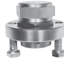
UTD450 Thermodynamic Steam Trap Module (Top Mount Style) Recommended for horizontal piping installations only so that cap can be oriented upwards as shown.
